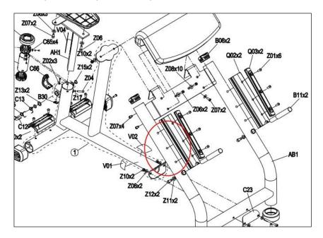
Below are the parts for the FW213 (A71) rework solution, **per side:** Q13 4pcs Z08 12pcs AB2 1pc
